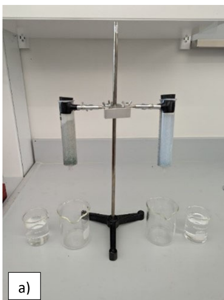
Fig. 5. a) Two syringes, each filled with a unique glass-bead size, fastened to a metal stand. b) Close-up of the open syringes and bead sizes (smaller on left, larger on right) before pouring water through the two mediums. Photo Credit: Masa Prodanović
